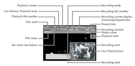
This unit displays the current recording/playback status by the bar meter. (Example of bar meter display)
